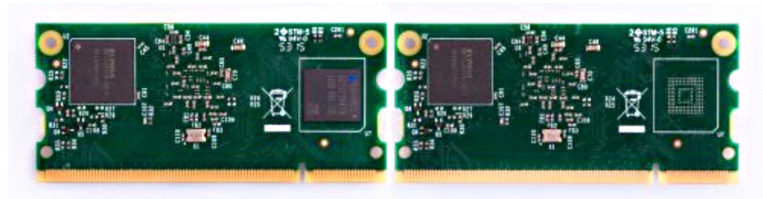
Back side of CM3 (left) and CM3L (right).
