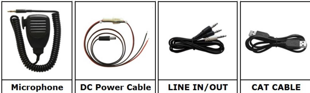
**Microphone:** An electrets mic that draws its power from the mic line (tip). If you use a dynamic mic, you must insert a 350 to 400 nF capacitor between the mic capsule and this line.
