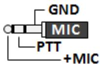
**PHONE:** The SKY-DSR accepts stereo headphones with a 3.5mm phone jack. Any common stereo headphones with an impedance of 4 to 64 Ohms will work; the lower the better.
