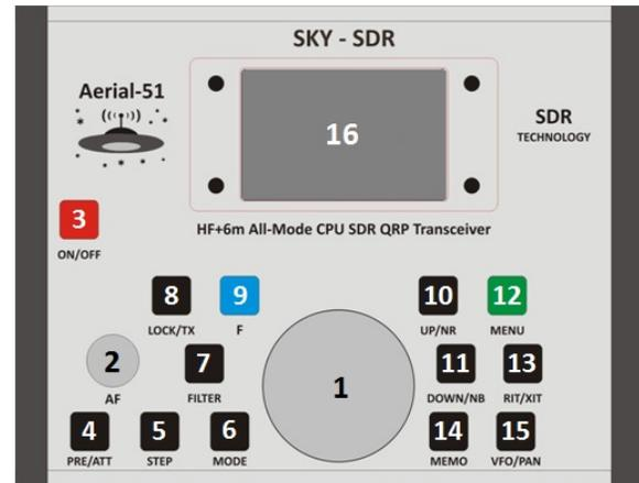
places the transceiver in transmit (TX) mode. Repeat the process to exit transmit mode and return to receive mode (RX).
