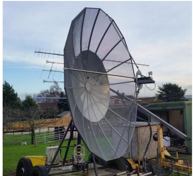
**M0MTS 3 m dish used in SSB Funtest with 300 W**
